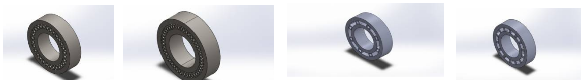
Fig. 3. (a) Hollow Circular core type vessel (b) Hollow ellipse core type vessel (c) Hollow Rectangular core type vessel (d) Rectangular core type vessel
